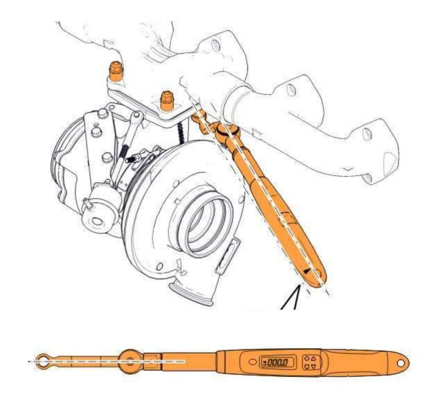
Apertar as porcas com o torque adequado.
